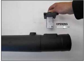
14. Install the mass air sensor assembly into the  $K\&N^{\circ}$  intake tube as shown, secure the sensor with the provided hardware.
