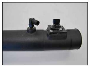
16. Install the 90° vent fitting into the K&N $^{\circ}$  intake tube as shown.
