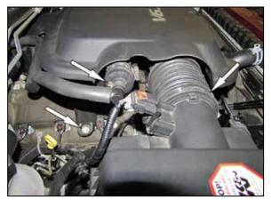
2. Loosen the hose clamp that secures the intake hose to the air filter housing. Using a screwdriver, unlock the small clamp that secures the vent line to the connector and then disconnect the vent line. Remove the bolt securing the intake plenum to the engine. 3. Remove the oil fill cap and loosen the hose clamp securing the intake hose to the throttle body. Remove the bolt securing the intake plenum to the engine.
