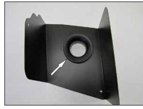
7. Install the filter adapter into the K&N<sup>®</sup> heat shield and secure with the provided hardware.
