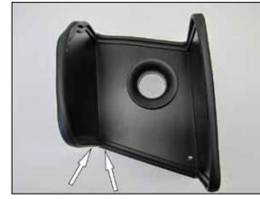
8. Install the edge trim onto the heat shield as shown.
