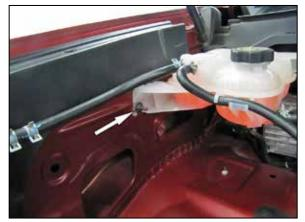
11. Remove the nut that secures the coolant reservoir to the inner fender. **NOTE: This nut will be reused in the next step.**
