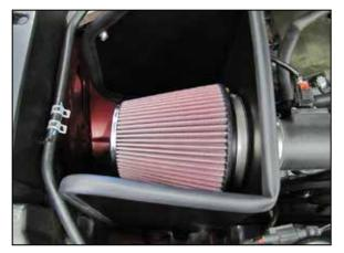
21. Install the K&N<sup>®</sup> air filter onto the filter adapter and secure with the provided hose clamp. NOTE: Drycharger<sup>®</sup> air filter wrap; part # RF-1042DK is available to purchase separately. To learn more about Drycharger<sup>®</sup> filter wraps or look up color availability please visit http://www.knfilters.com<sup>®</sup>.
