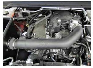
18. Install the provided hump coupler (08699) onto the K&N<sup>®</sup> intake tube, then install the intake tube assembly into the coupler at the throttle body and align with the filter adapter. Slide the hump coupler onto the filter adapter, adjust the tube for best fit and secure with the provided hose clamps.
