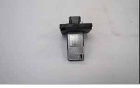
13. Remove the mass air sensor from the factory air filter housing and install the sensor and provided gasket into the K&N<sup>®</sup> mass air sensor adapter using the provided hardware.
