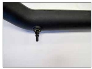
17. Install the quick connect fitting into the  $K\&N^{\circledast}$  intake tube as shown.
